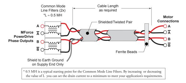
Figure 2.3.8: Motor Cableing Greater than 50 Feet
